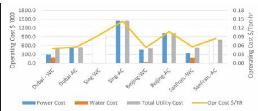
FIGURE 6. Operating cost, power, and water-heavy load profile.
