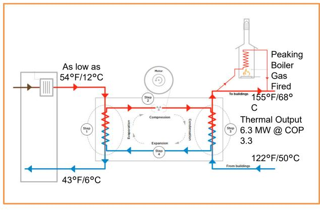
Fully packaged high temperature high lift centrifugal heat pumps will provide **155°F/68°C heating water** (21,500 MBH/6.3 MW) for connected buildings
