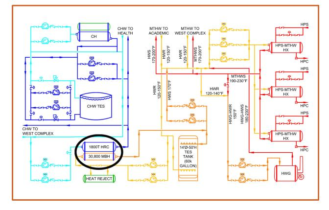
Conversion from medium pressure steam and high temperature hot water to low temperature hot water
